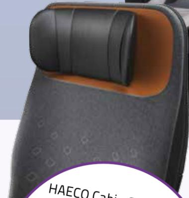
HAECO Cabin Solutions created a double-hinge headrest to support the head and neck better than static and articulating headrests. Arc has a five-segment, articulating-joint cushion system with adjustable tilt and height
